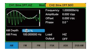
The T3AFG range of Function/Arbitrary Waveform Generators support a wide range of modulation types including AM, FM, PM, FSK, ASK, PSK, PWM and DSB-AM.
